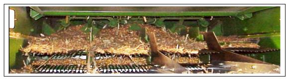
If they are not evenly filled, balance out the shoe evenly by adjusting the auger bed deflectors or adding round bar concave sectionalized covers.
